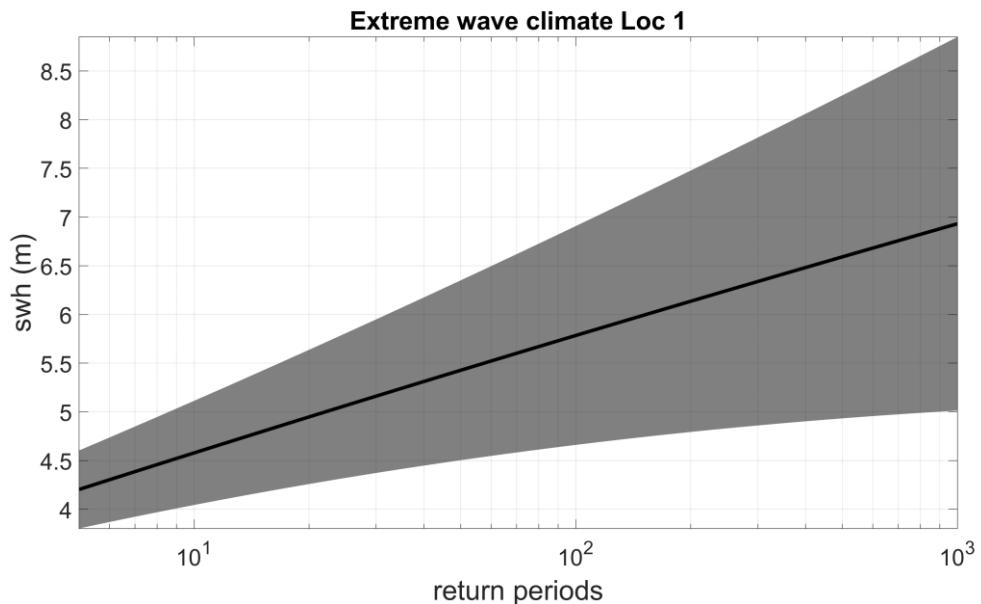
The time series is too short to be compute larger return period, this can be seen in the large confidence interval. Let's compare the plotted results with a proper lime series longer enough to minimize the error for the longer return period.
